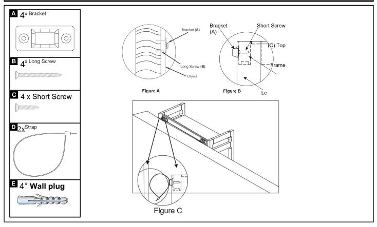
Using a second person to assist you, place the unit in the desired final location against a wall. It is suggested to use a stud finder to find wall studs along the length of the unit and roughly 1 inch below the top of the unit. Where possible, mark a drill hole position on the wall where there is a stud and use a drill or screwdriver (NOT INCLUDED) to attach wall Brackets (A) to the wall using Long Screws (B) in the location of the wall studs.
