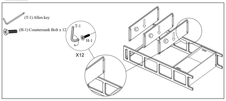
Carefully position each Shelf (C) onto the top, middle and bottom positions. Secure with Countersunk Bolts (H-1) through each cleat beneath the Shelves (C) into the Right/Left Legs (A/B). Engage until snug, but DO NOT YET FULLY TIGHTEN.
