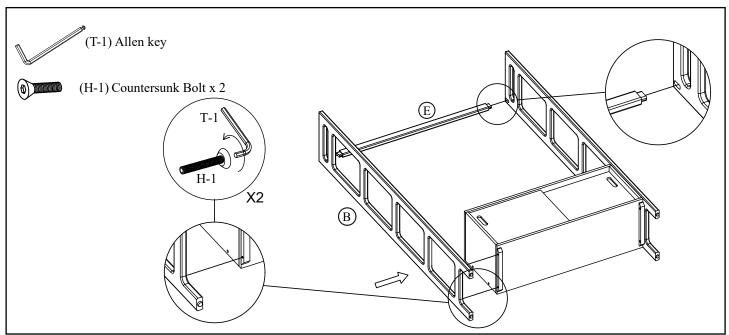
Insert the end of the Top Support (E) into the mortise at the top of the Right Leg (A) from step 1. Position the Left Leg (B) on the other side of the Cabinet (D), and at the same time insert the other end of the Top Support (E) into the mortise. Insert and engage the Countersunk Bolts (H-1) at each connection point inside and on the bottom of the cabinet with the receiving holes on the Left Leg (B). Tighten the hardware until they are snug, but DO NOT YET FULLY TIGHTEN.
