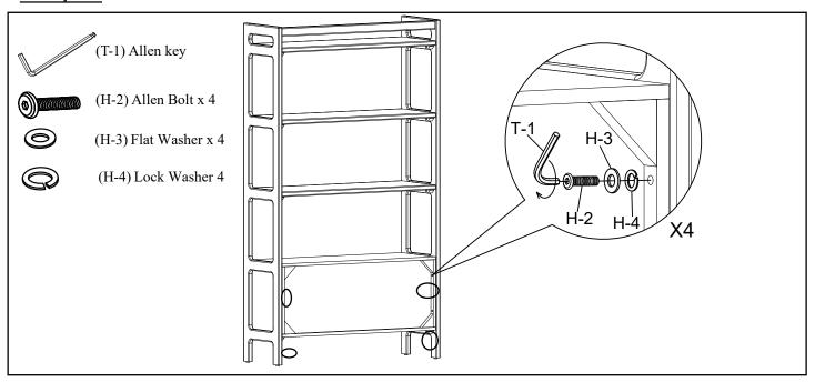
Using a second person to assist you, carefully position the entire assembly upright. Secure the back of the Right/Left Legs (A/B) to the Cabinet (D) by engaging Allen Bolts (H-2), Flat Washers (H-3) and Spring Washers (H-4) through the back frame of the Cabinet (D), stacking the hardware in the order as shown. Now fully tighten ALL hardware from this and previous steps using the provided Allen Key (T-1). DO NOT OVER TIGHTEN.
